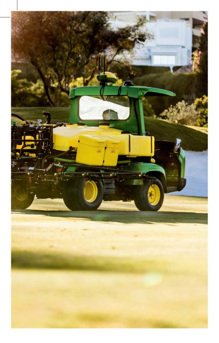
Based on the established combination of a ProGator™ utility vehicle and HD200 low profile sprayer, the new 750-litre capacity GPS PrecisionSprayer offers a proven, off-the-shelf, integrated solution for precision spraying on amenity turf.
